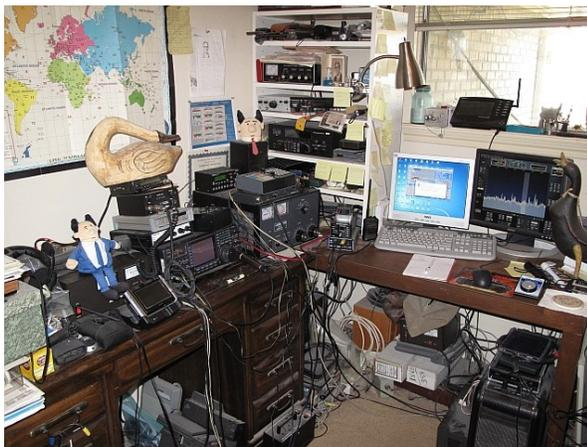
Lately he has become interested in QRP operation. He has an Elecraft KS-1 and a Flexradio Flex 1500 which has aroused an interest in Software Defined Radio. He also has an Icom IC-756 and an Ameritron AL-572 which he admits to cranking up when conditions are not so good for QRP. He has a Yaesu FT-857 with an ATAS-120 in his car so he can pass the time while stuck in traffic.
