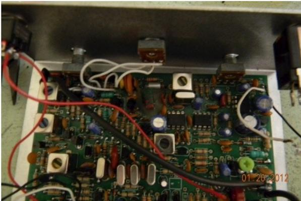
The reason was this little plug.. The big Polystyrene cap (seen in the middle of the photo, nearly white in color and lying behind the middle pot). This HO16 quit working and had to be replaced. Well
