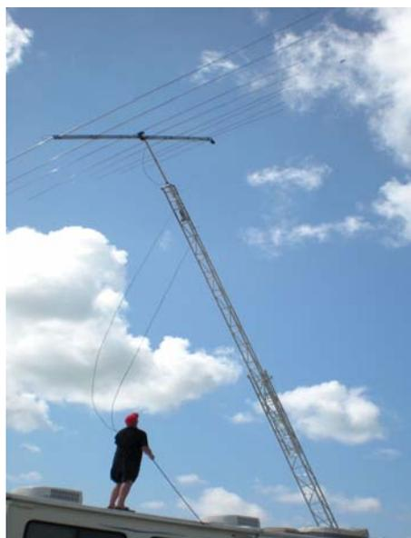
Our HF antenna was a tribander at 35 feet on a crankup tower, permanently mounted on the motorhome. Just driving out the dike and listening on 20m, signal's went from, say s4 to S8 by the time I arrived at the site...
