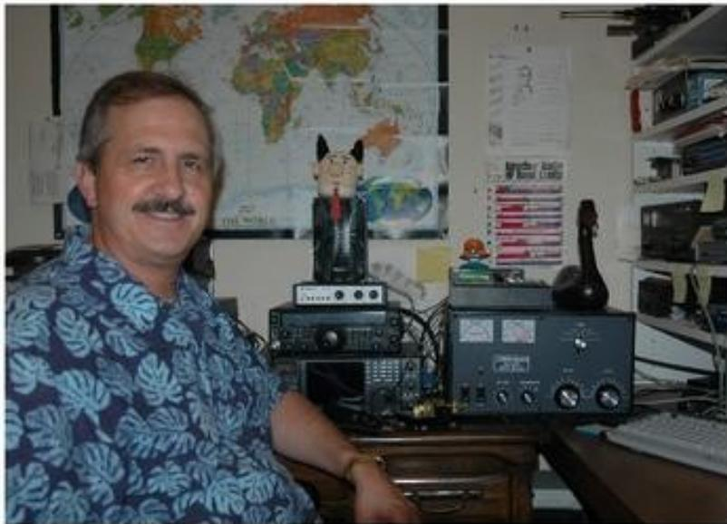
That's an ICOM 756 Classic and a Yaesu FT-847 with an Ameritron AL-572 amp. Now there's also a tiny Flex 1500 SDR as well. Antenna outside is a SteppIR Big Vertical.
