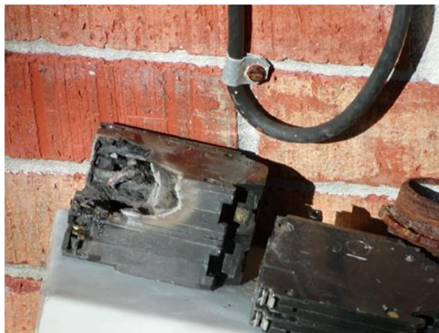
This is the circuit breaker that failed and burned up my feed panel. The coax is my computer modem feed which just happens to be in the picture.
